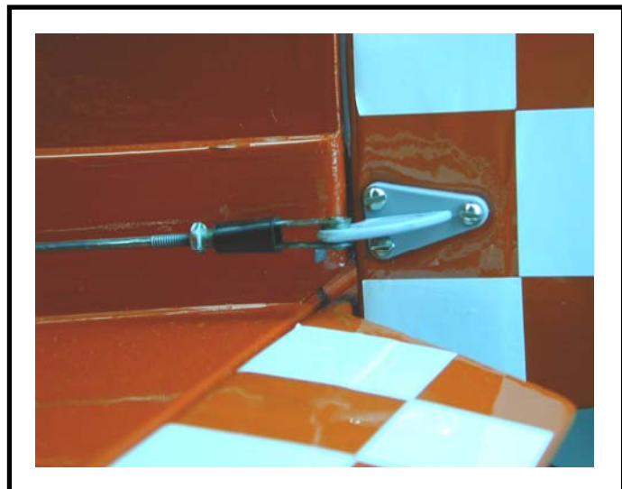
A secure, tight, non-binding horn linkage.
